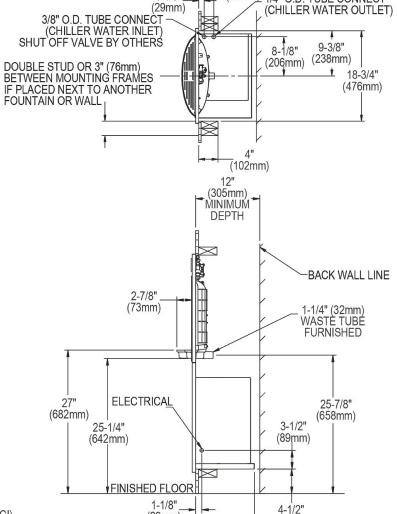
Note: New Installations Must Use Ground Fault Circuit Interrupter (GFCI). (29mm)11" It is highly recommended that the circuit be dedicated and the load protection be sized for 20 amps. (279mm)
